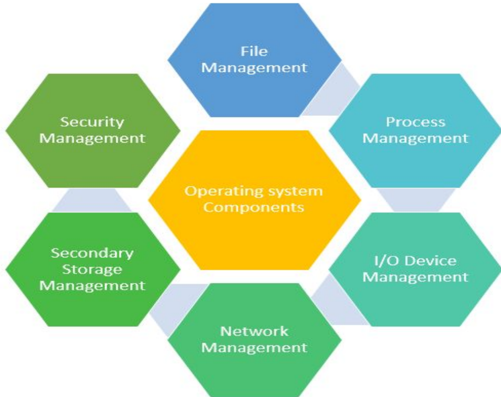
Fig. 1 : Operating System Components
