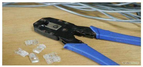
**Step 3.**Cut the cable to length. Determine the length needed for your cable and use the wire cutting tool on the crimping tool to cut the cable to this length.
